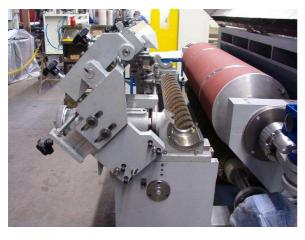
In the **new project** we have improved the roller buffing machine by including all new devices studied for the belt buffing machine and we have **standardised the main components** like feed roller high precision control, the high resistance feed roller shaft, , the combined grip roller and grip blade system, the separate drive of buffing brush etc., to get highest performances and matchless **reliability under heavy work conditions**.
