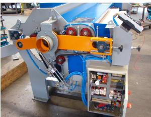
The dust-removing machine is provided by **adjustable feeding speed** in order to be synchronised with any kind of buffing machine. Even the height of the front feeding belt can be adjusted within a wide range, so that every buffing machine can be installed before our dust-removing machine, without need of particular adjustments.
